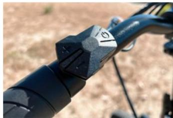
The IF module and Thumb Controller were an innovation required to “clean up” the bike handlebars. Our prospective customers demanded that we not clutter them with loads of devices. In this case, we could remove the typical display and Thumb Controller used on most eBike with the KSS App and the IF module and compact Thumb Controller. This offered one single display in front of the rider.
