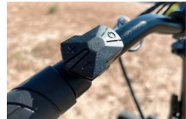
The IF module and Thumb Controller were an innovation required to “clean up” the bike handlebars. Our prospective customers demanded that we not clutter them with loads of devices. In this case, we could remove the typical display and Thumb Controller used on most eBikes with the KSS App and the IF module and compact Thumb Controller. This offered one single display in front of the rider.
